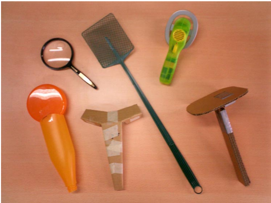
Figure 21: Shapes scavenged and constructed to explore possible forms for a hand-held locator.
