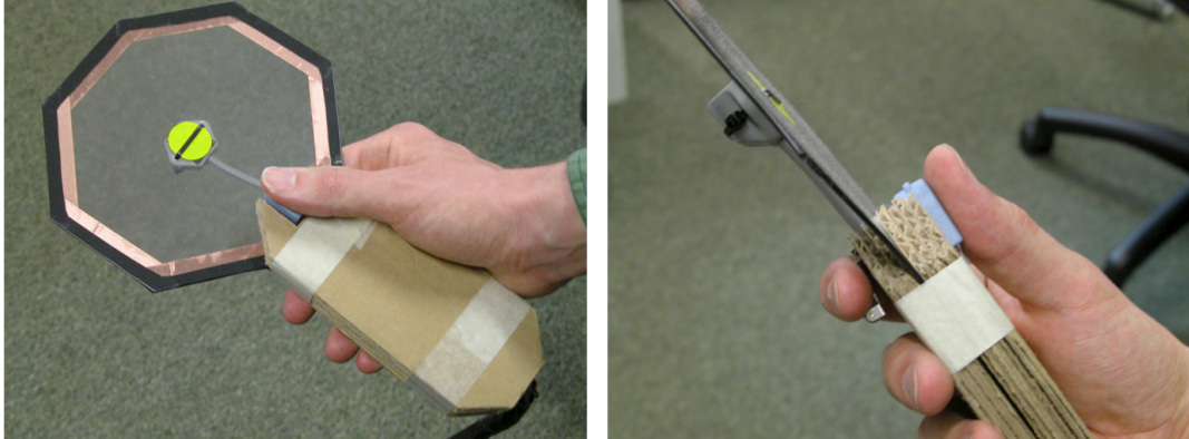
Figure 22: Left: The hand-held locator's final form. Right: A close-up illustrating the locator's active elements: a vibrotactile transducer (under thumb), a button (activated by one's trigger finger) and the Fastrak position sensor (visible to the upper-left).
