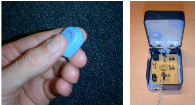
Figure 17: Left: The VBW32 transducer used for vibrotactile display. Right: A custom amplifier used to boost the power of the signal delivered to the transducer.
