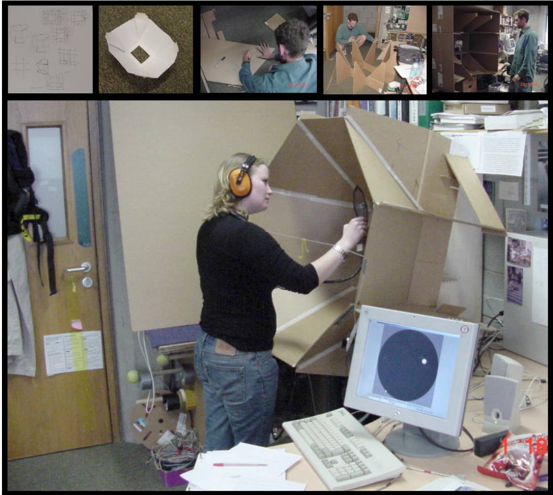
Figure 29: Actual experimental apparatus and environment. Top: Sketches, paper models and construction of the search volume. (The idealized hemispherical search volume was realized as a multifaceted cardboard construction). Bottom: Participant within the experimental environment, engaged in locating a target in the search volume.
