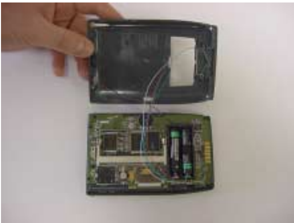
Figure 21: PDA being wired
